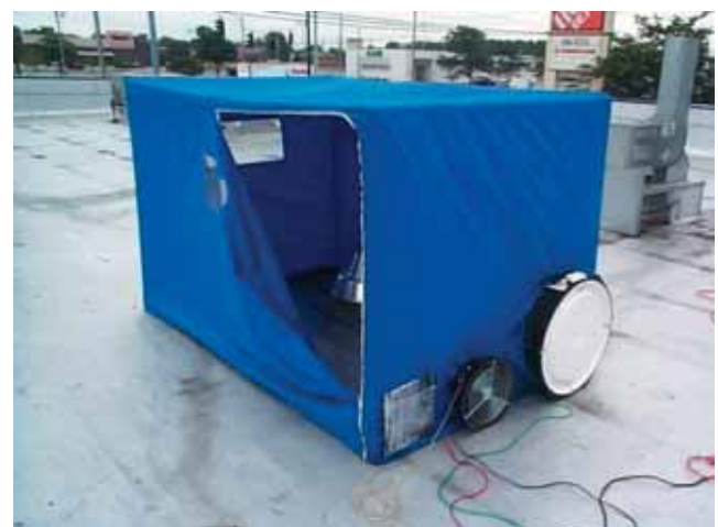
Figure 7 - Fan powered capture hood measuring flow from a rooftop exhaust fan. This method provides good accuracy but is limited to flows equal to or less than the flow of the calibrated fan. Photo courtesy of CDH Energy Corporation and New York State Energy Research and Development Authority.
