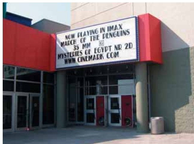
Figure 2 - Multiple blower doors used in buildings with leakage areas too large for a single blower door.
